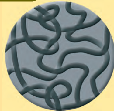
Figure 11: Random, Non-Symmetrical Chains
