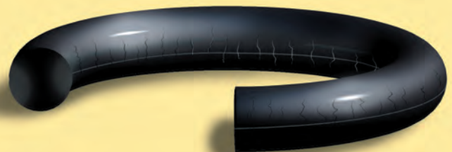
Figure 138: Failure Due to Weather & Ozone Cracking
