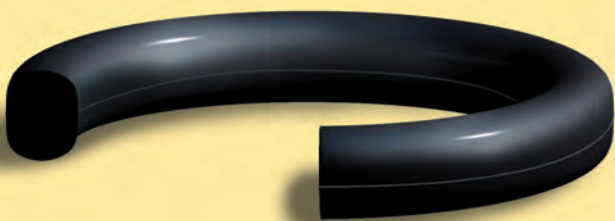
Figure 129: Failure Due to Compression Set
