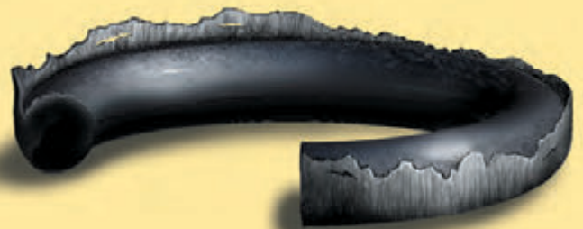
Figure 132: Failure Due to Extrusion & Nibbling
