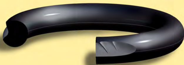
Figure 135: Failure Due to Installation Damage
