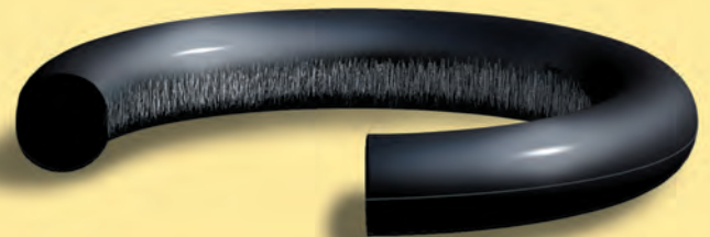
Figure 128: Failure Due to Abrasion
