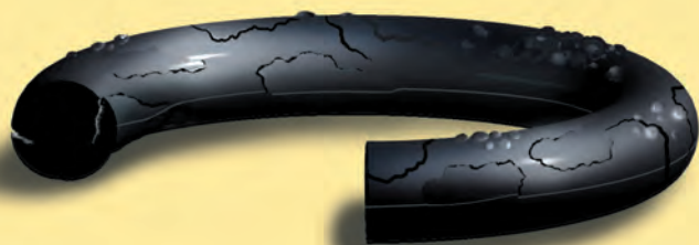
Figure 131: Failure Due to Explosive Decompression
