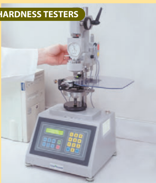
Figure 15: Some instruments can generate both durometer and IRHD readings.
