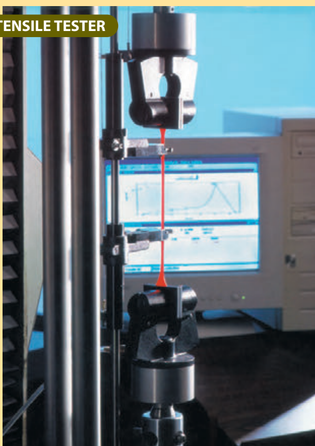
Figure 18: Stretching a Sample
