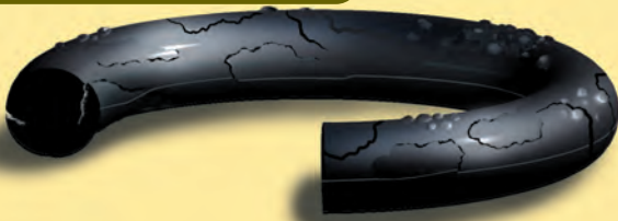
Figure 55: Failure due to explosive decompression.
