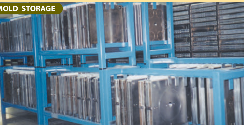
Figure 156: Individual mold plates are organized for easy retrieval.
