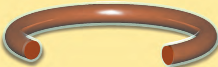
Figure 145: Fluoroplastic jacket around a silicone core.
