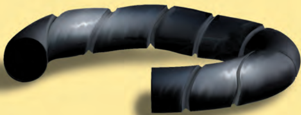
Figure 137: Failure Due to Spiraling
