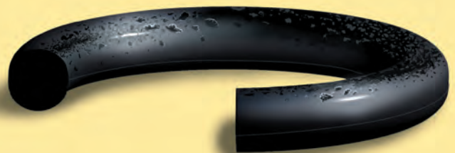
Figure 130: Failure Due to Dieseling
