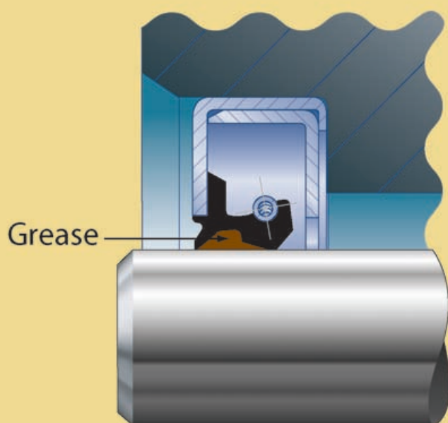
Figure 177: Provides Seal & Shaft Lubrication
