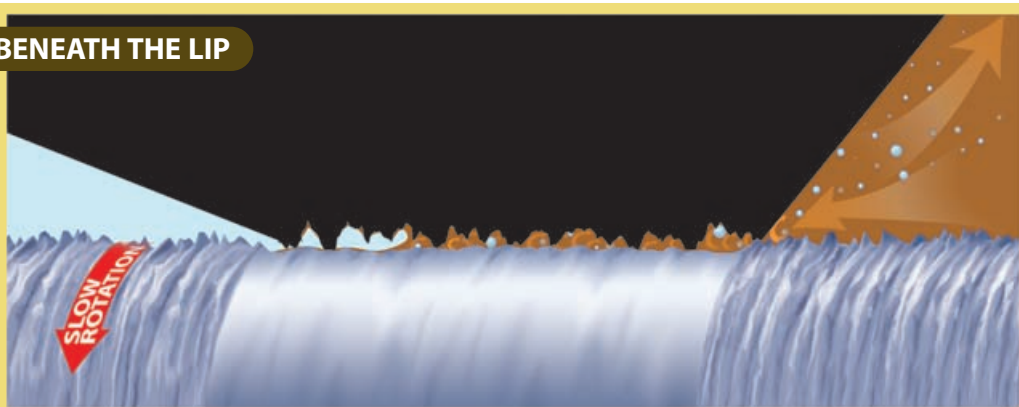
Figure 146: Microasperities Assist Underlip Fluid Pumping
