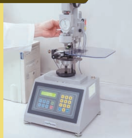
Figure 16: Some instruments generate both durometer and IRHD readings.
