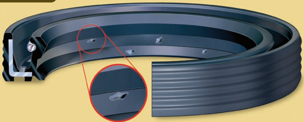
Figure 157: Irregular Surface Protrusions
