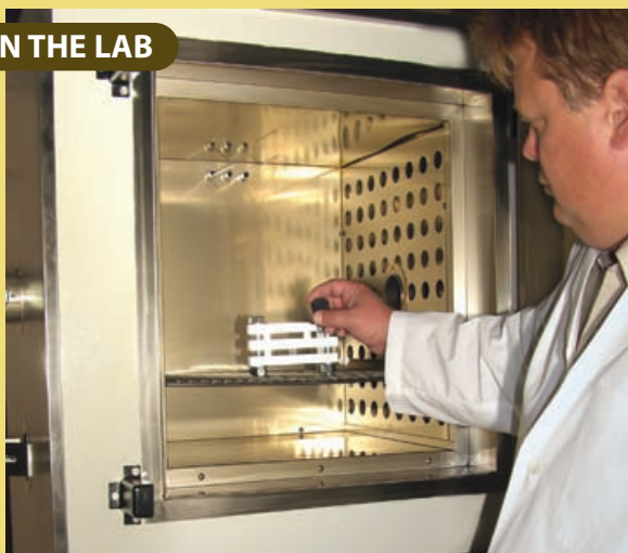
Figure 43: Our Blue M oven and specialized test fixtures allow for compression set testing.
