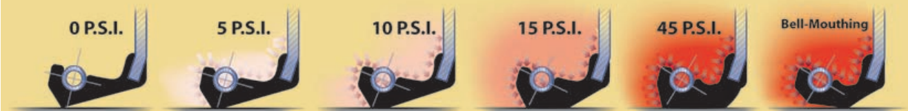
Figure 187: Effects of Pressure on Standard Shaft Seal Lip
