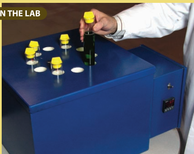
Figure 44: Our heating block provides us with precise temperature control during fluid resistance tests.
