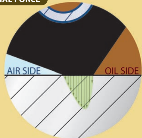
Figure 142: Contact Pressure Distribution Pattern
